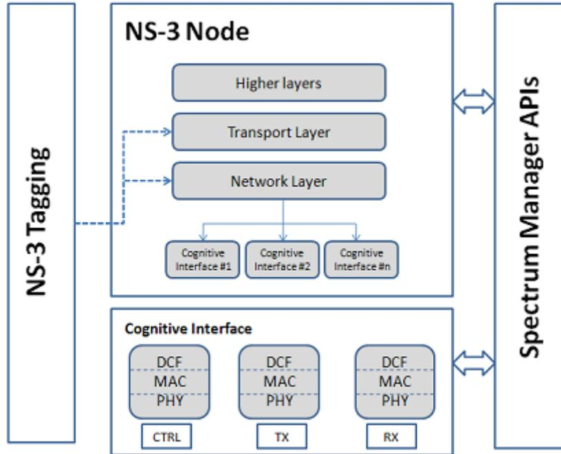
Figure 2: Layered Architecture of an NS-3 CR Node
